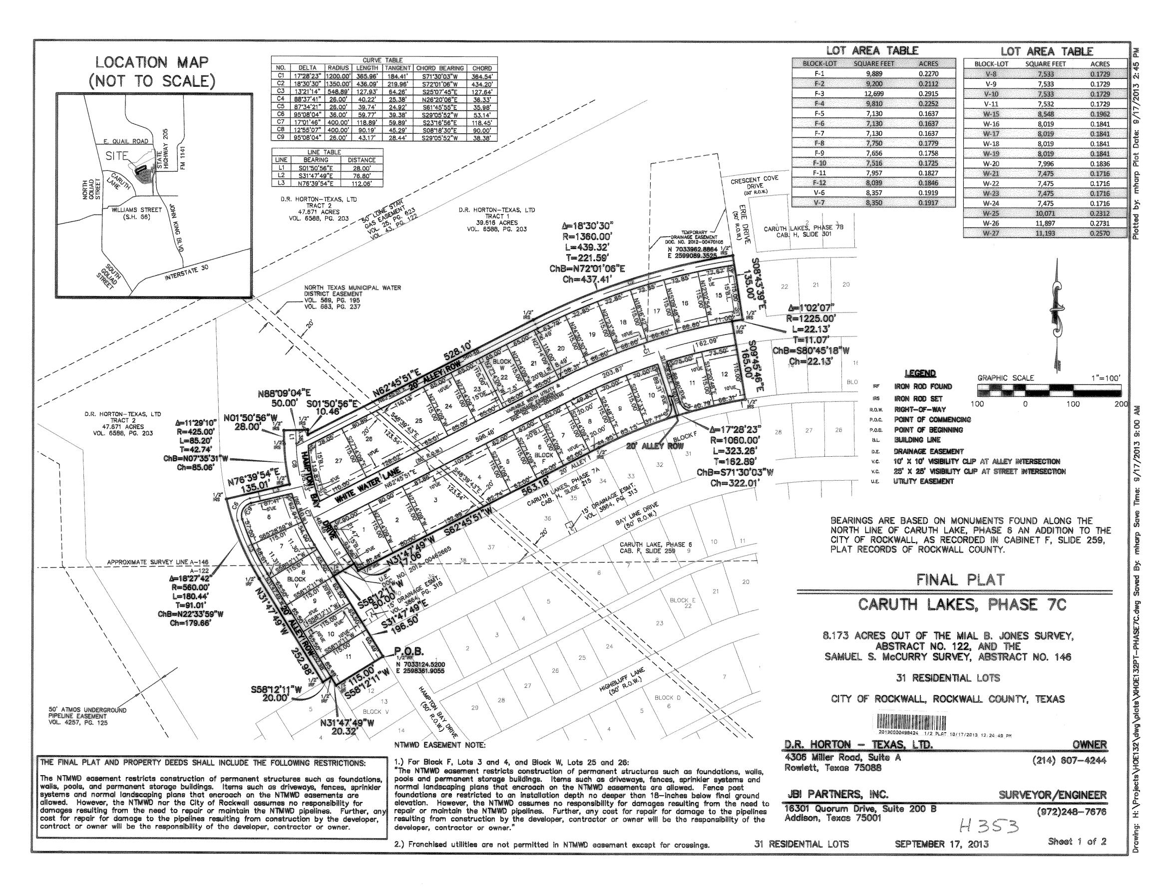
BEGINNING at a one-half inch iron rod found in the south line of said Tract 1. said point being the north corner of Lot 12, Block V, Caruth Lake, Phase 6, an addition to the City of Rockwall as recorded in Cabinet F, Page 259, Plot Records of Rockwall County, said point also being in the southwest right-of-way line of Hampton Bay Drive (a 50 foot right-of-way) dedicated by said Caruth Lake, Phase 6 plat;
