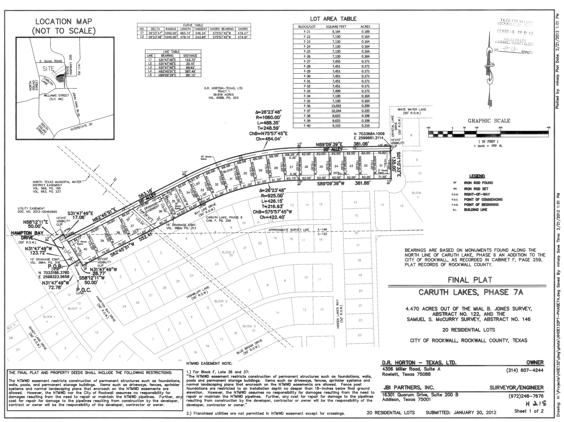
COMMENCING at a one-half inch iron rod found at the north corner of Lot 12, Block V, Caruth Lake, Phase 6, an addition to the City of Rockwall as recorded in Cabinet F. Page 259, Plat Records of Rockwall County, said point also being in the southwest right-of-way line of Hampton Bay Drive (a 50 foot right-of-way) dedicated by said Caruth Lake, Phase 6 plat:
