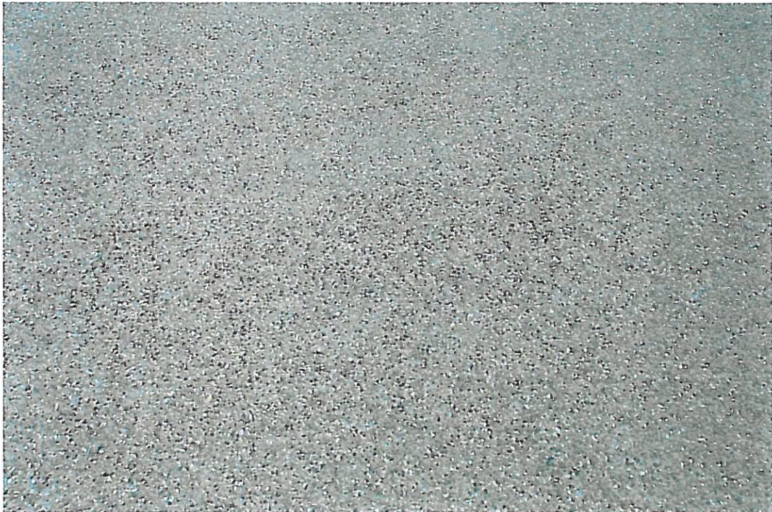
Proposed look of exposed aggregate concrete.
