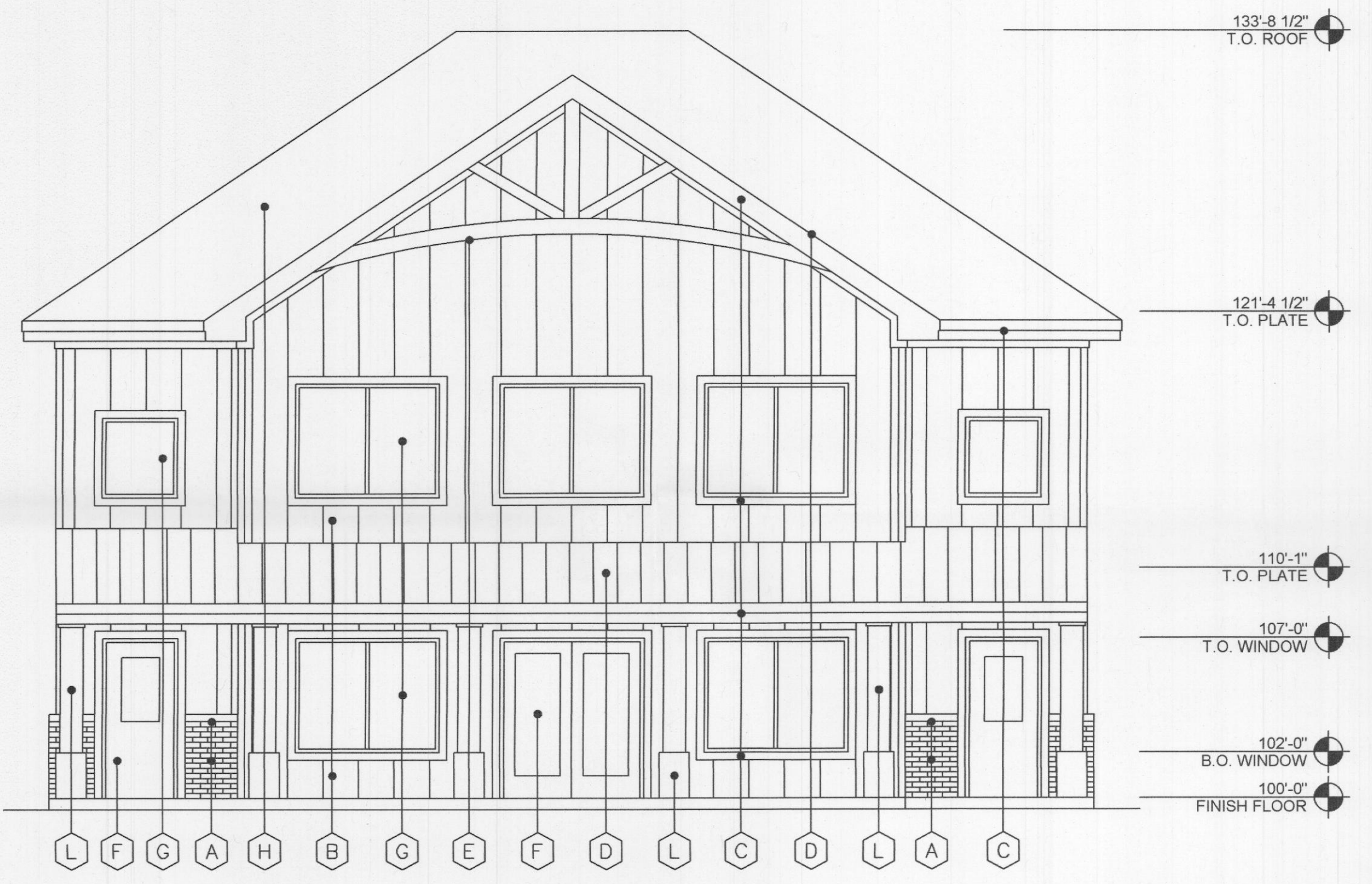
3 WEST ELEVATION - MASONRY: 6% SCALE: 3/16" = 1'-0"
