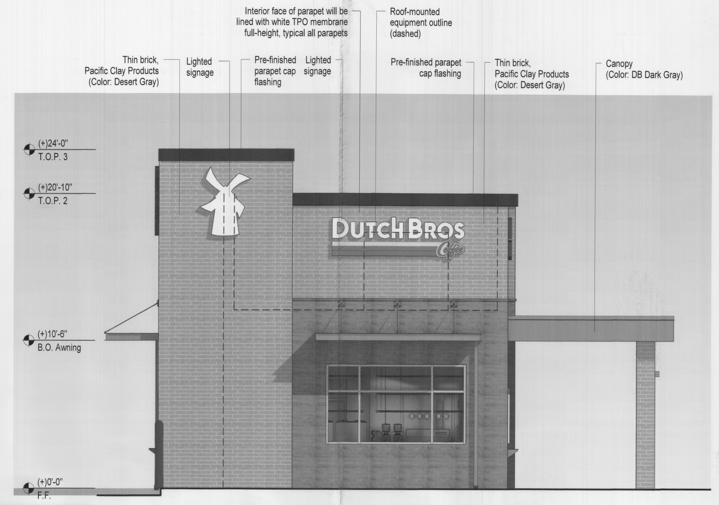
East Elevation - (Front Elevation) 1/4" = 1'-0"
