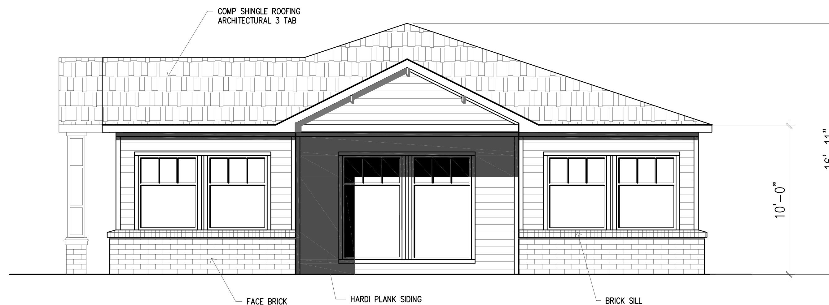
NORTH ELEVATION 100% MASONRY 34% STONE 66% HARDI PLANK
