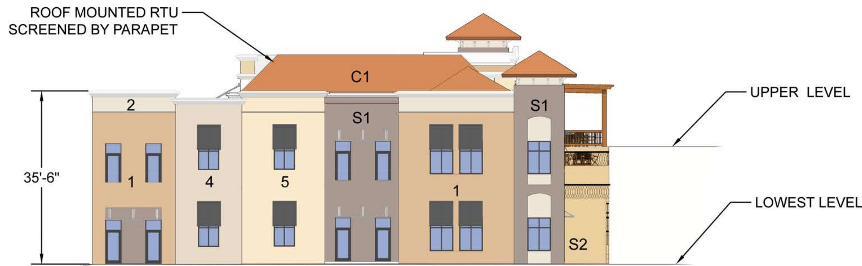
3 WEST ELEVATION SCALE: TOTAL BUILDING WALL HARD SURFACE : 3,616 SF TOTAL PLASTER: 2,857 SF = 79% TOTAL BUILDING STONE: 759 SF = 21%
