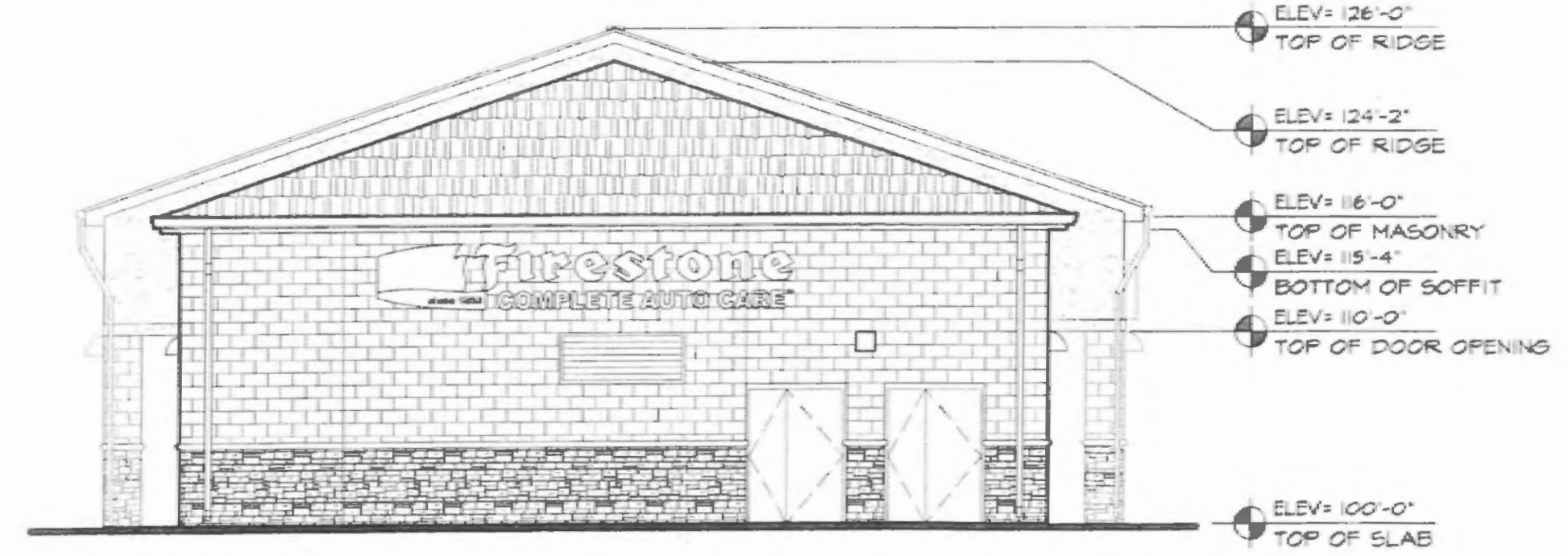
02 NORTH ELEVATION 1/8"=1'-0" I-30 & WHITE HILLS DRIVE
