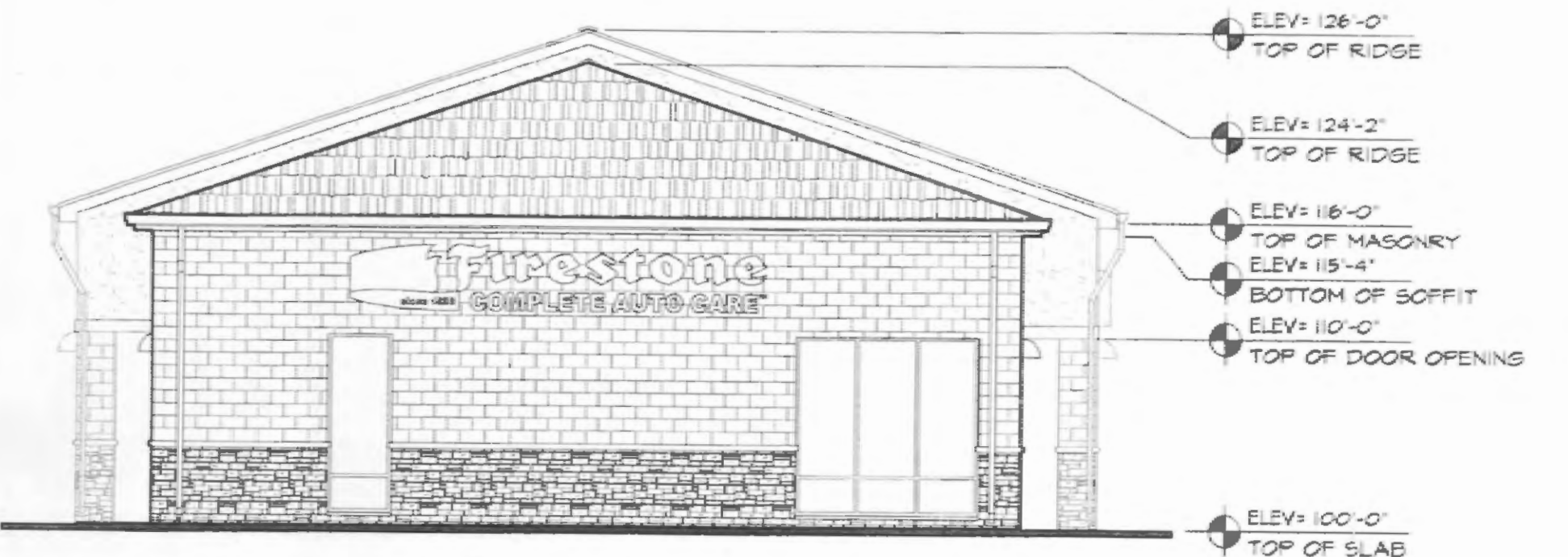
03 SOUTH ELEVATION 1/8"=1'-0" I-30 FRONTAGE
