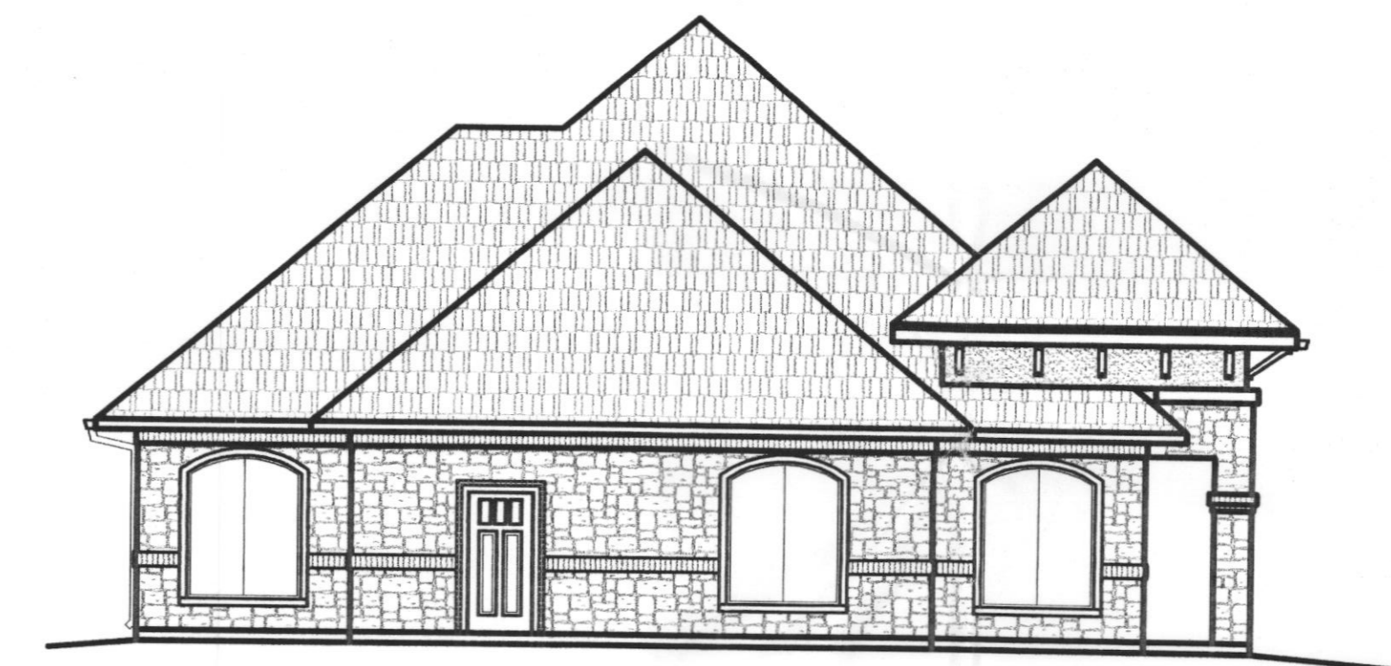
2 building elevation - side scale: 1/8" = 1'-0"
