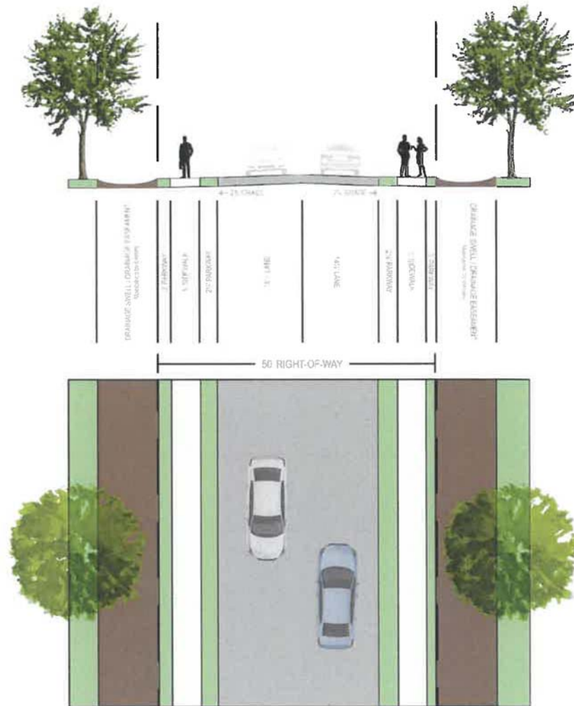
Figure 3: Rural-Local Roadway Cross-section
