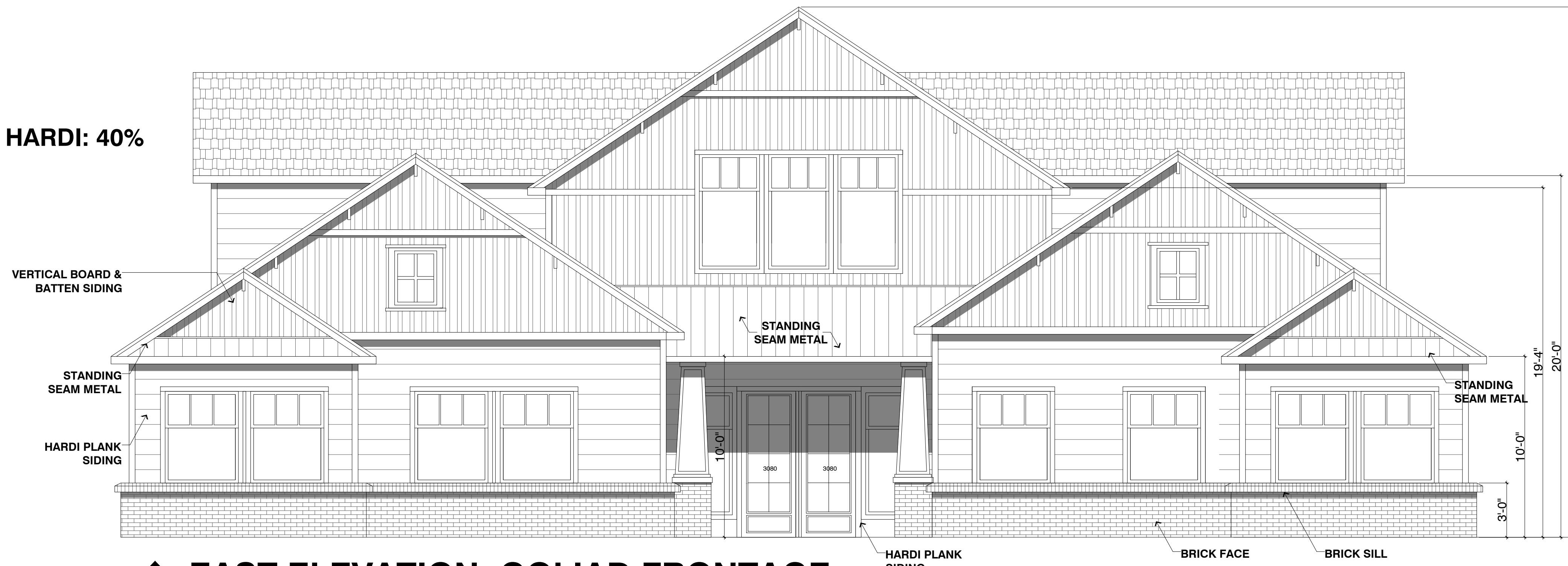
301 EAST ELEVATION: GOLIAD FRONTAGE SCALE: 1/4" = 1' - 0"
