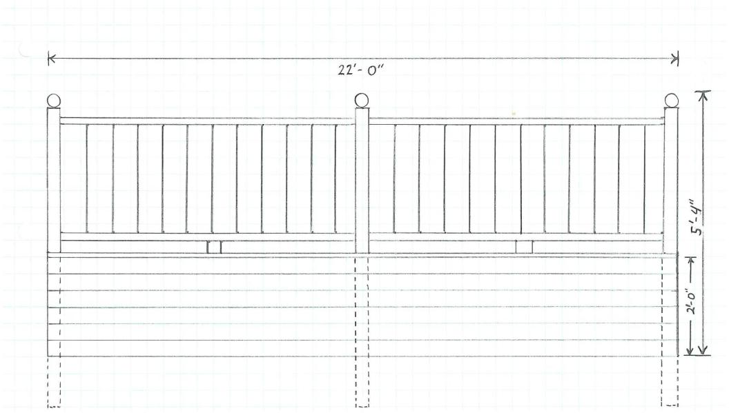
TOP VIEW SHOWN. SUPPORT POST TO BE 4"x4" CONCRETED IN THE GROUND, FRAMING MATERIALS TO BE 2x8". DECK, BOARDS TO 2"x6". ALL MATERIALS TO BE PRESSURE TREATED.
