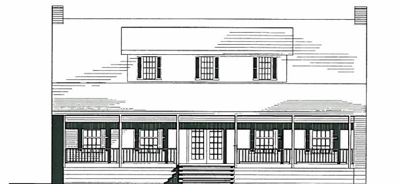
NEW RESIDENCE WEST ELEVATION
