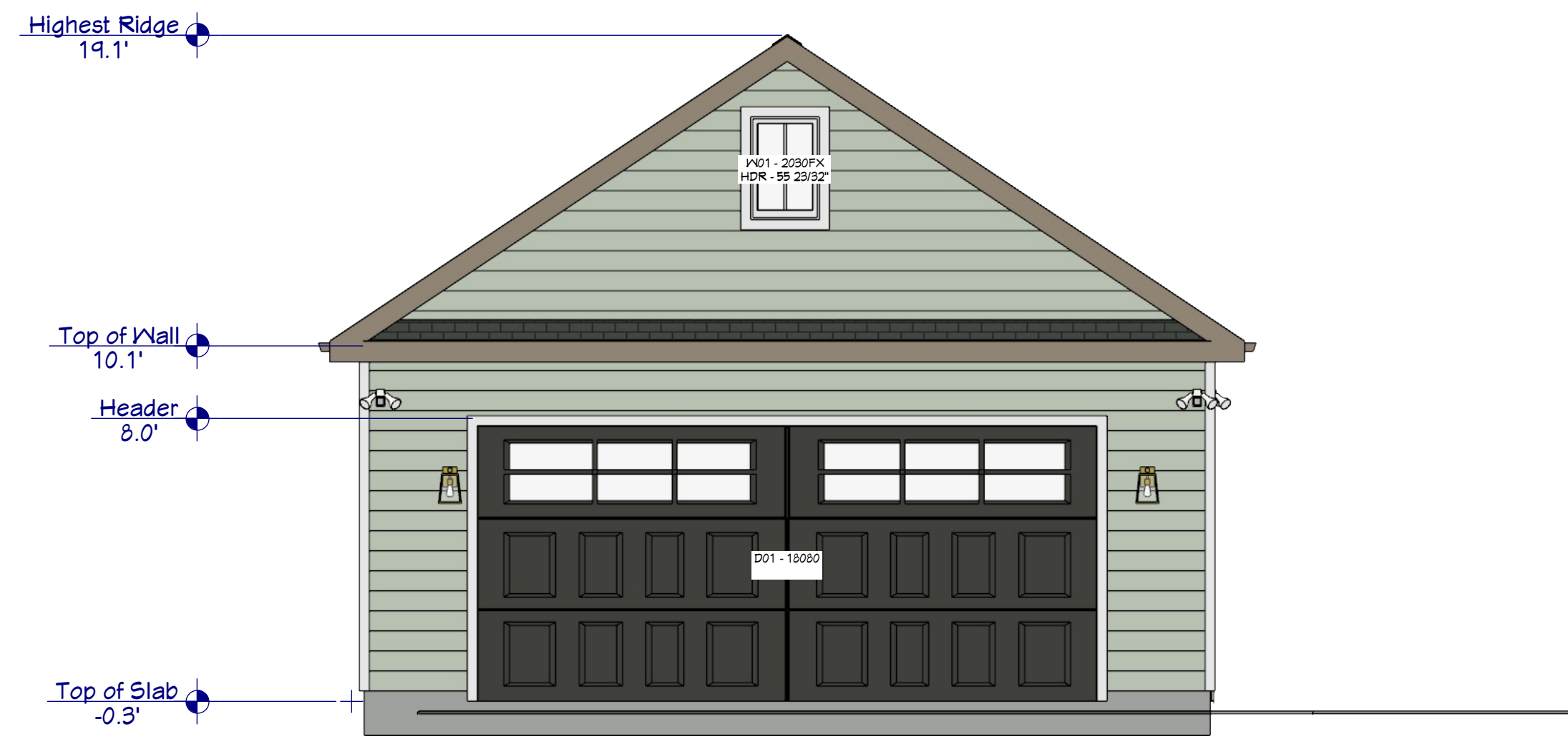
Exterior Elevation Front
