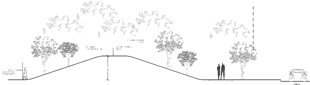
FIGURE 10. TYPICAL CROSS SECTION OF LANDSCAPE BUFFER FOR JOHN KING BOULEVARD
