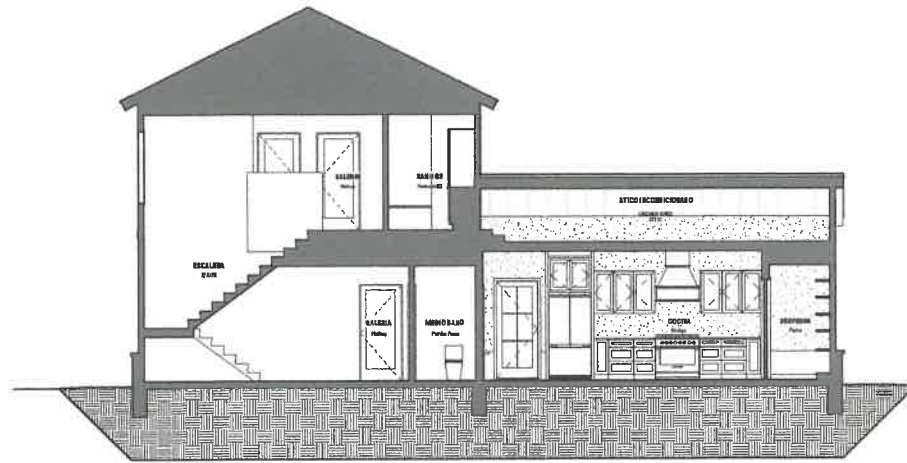
02 | BUILDING SECTION AT KITCHEN AND STAIRS 302-101-101
