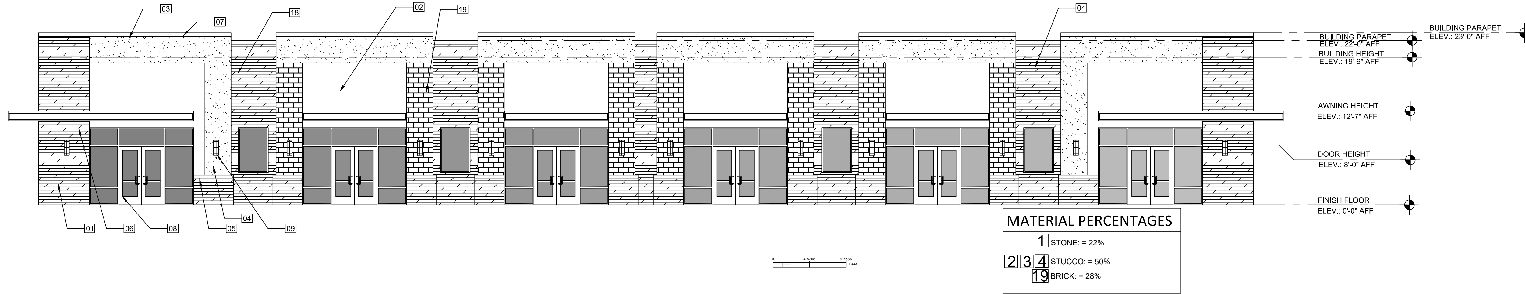
01 FRONT ELEVATION Scale 1/8" = 1' - 0"
