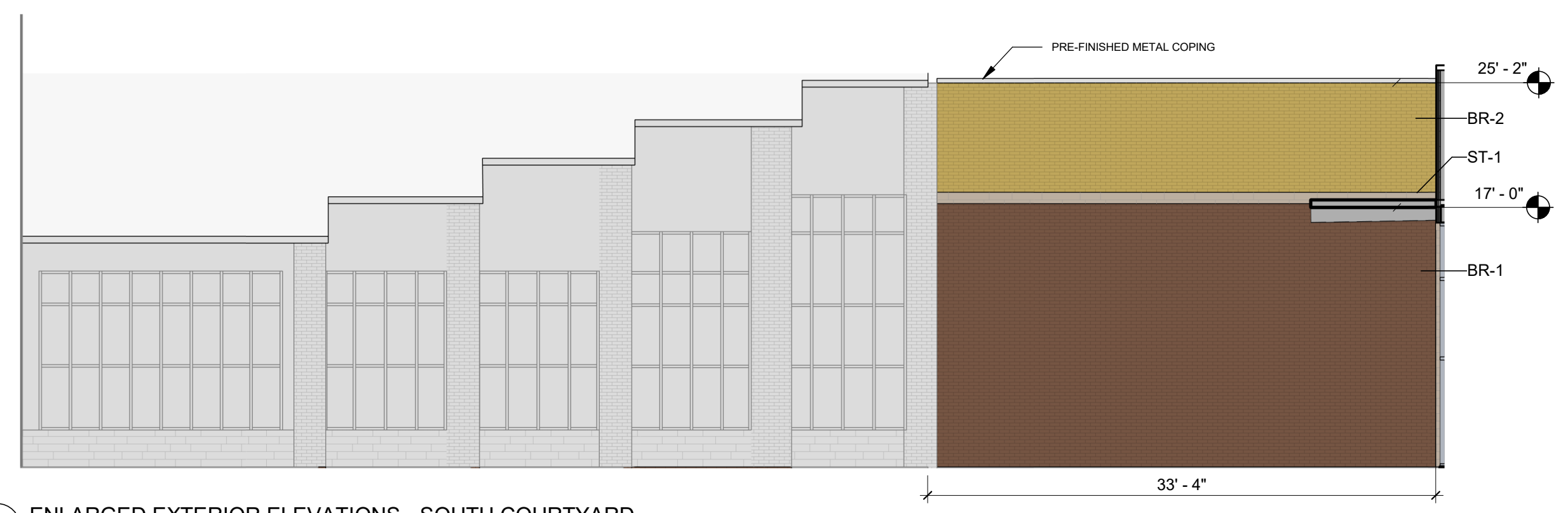
02 ENLARGED EXTERIOR ELEVATIONS - SOUTH COURTYARD 1/8" = 1'-0"
