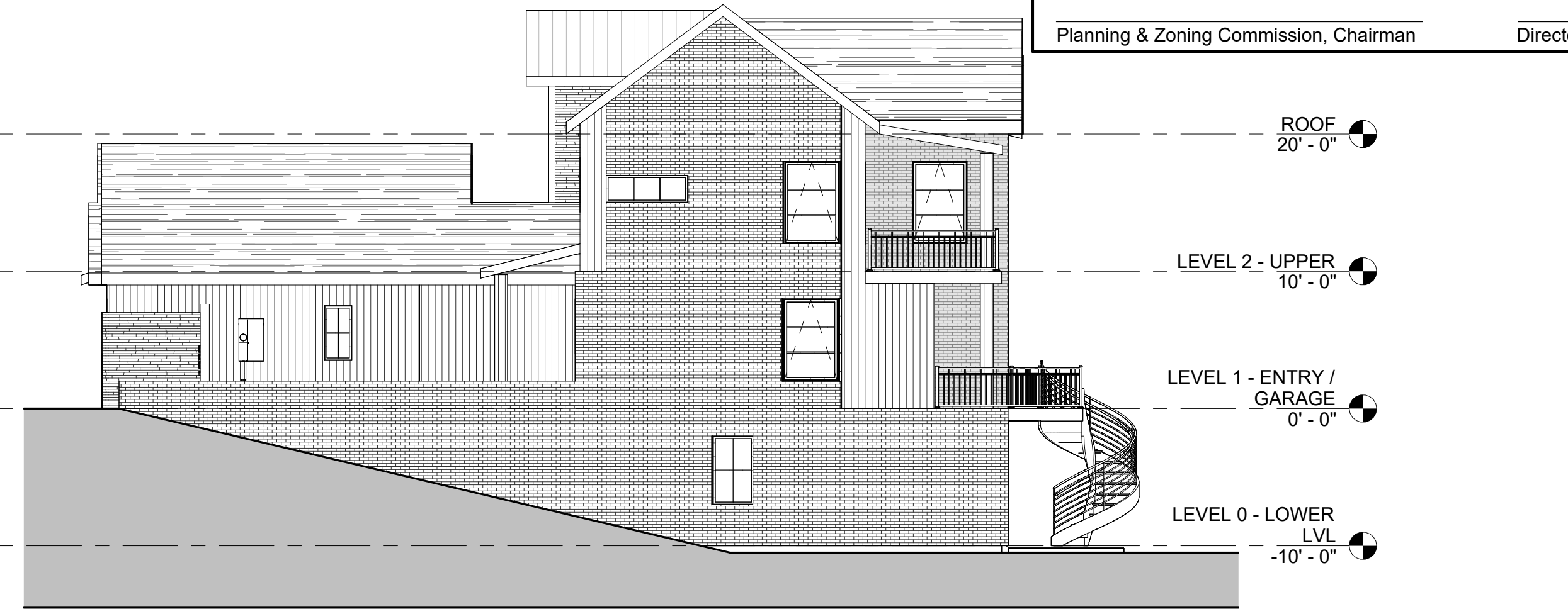
3 RIGHT SIDE ELEVATION 1/8" = 1'-0"
