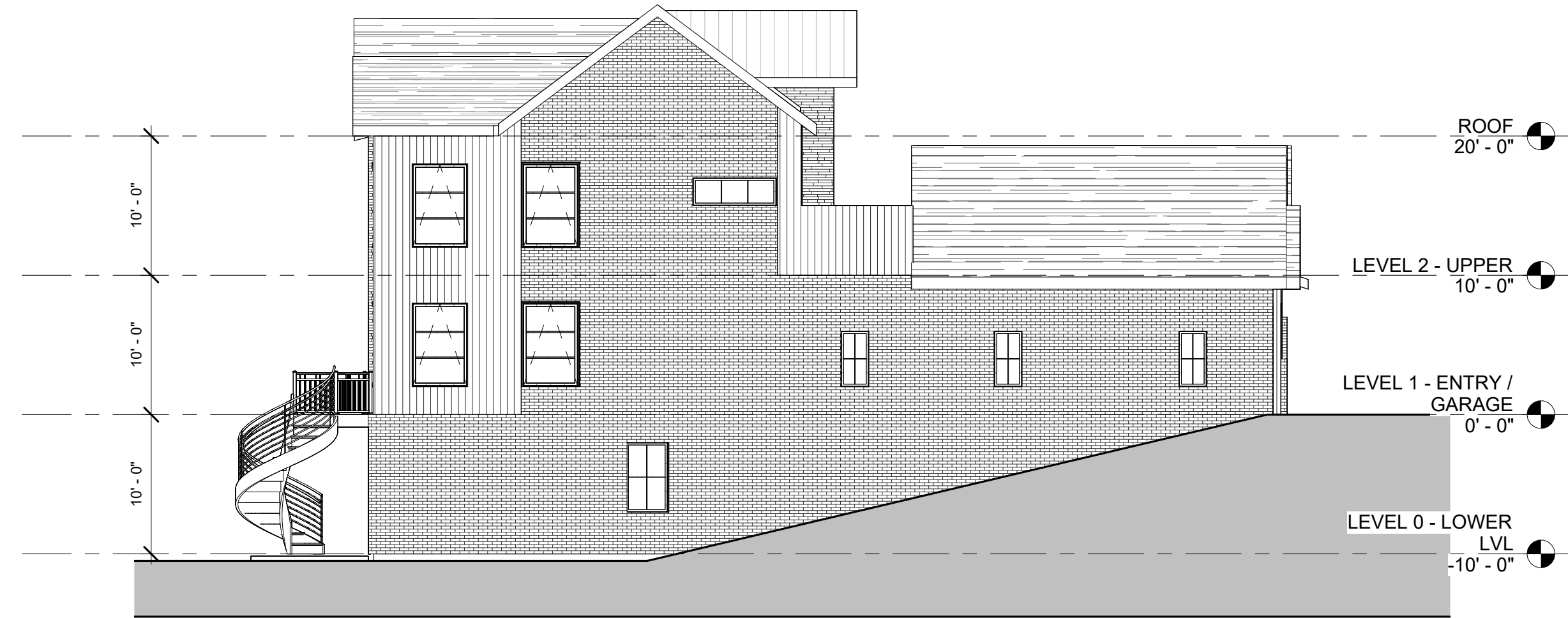
4 LEFT SIDE ELEVATION 1/8" = 1'-0"
