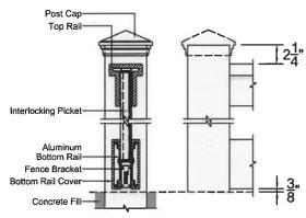
Post Profile: Cut View / Elevation View
