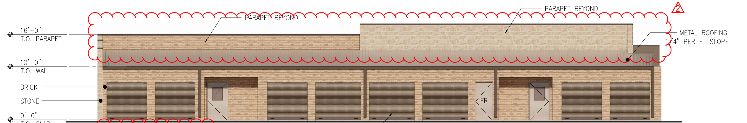
BLDG D WEST ELEVATION SCALE: 3/32" = 1'-0"
