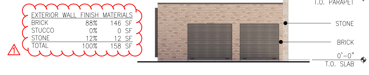
BLDG C SOUTH ELEVATION SCALE: 3/32" = 1'-0"
