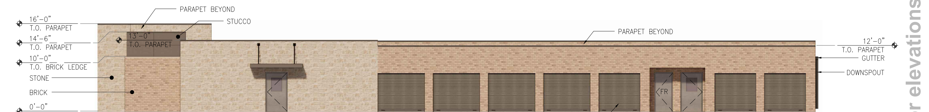
BLDG B SOUTH ELEVATION SCALE: 3/32" = 1'-0"
