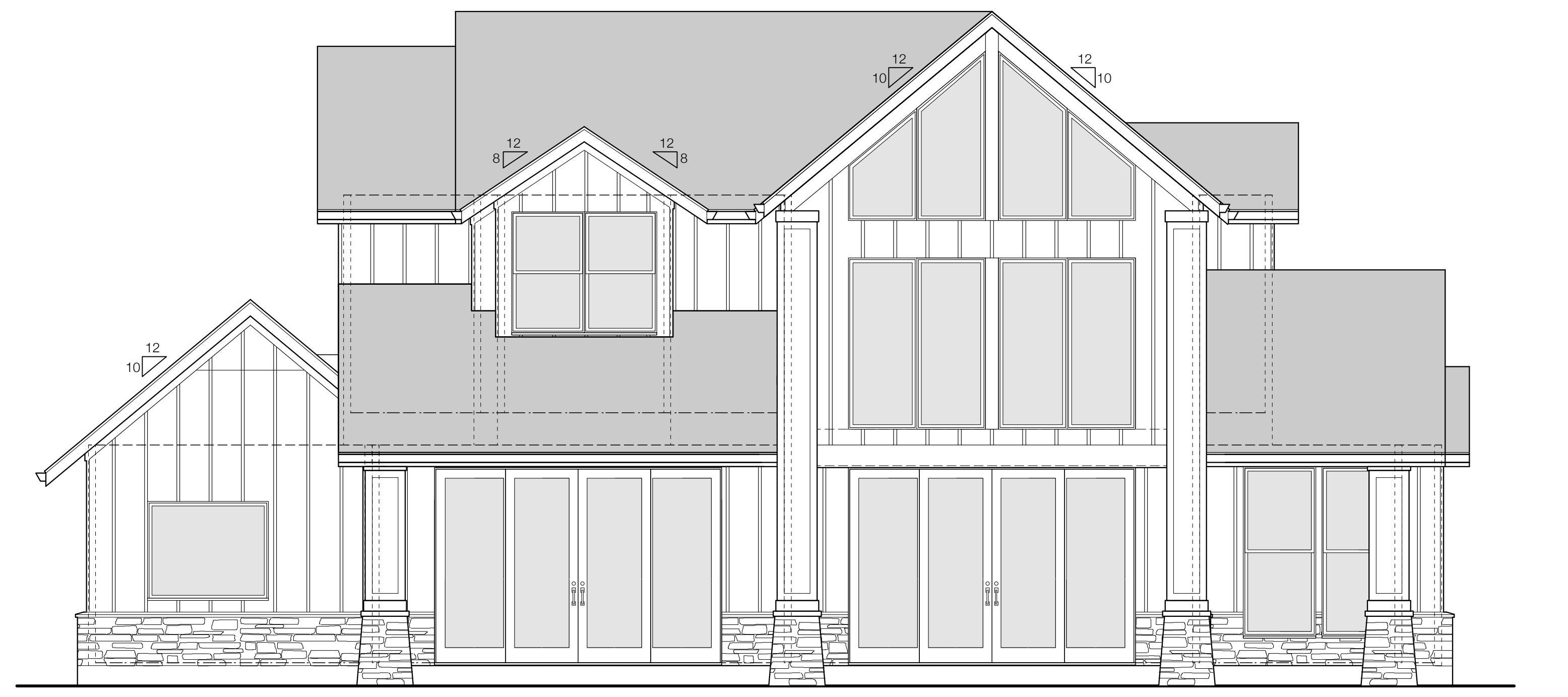
01 3.01 GUEST HOUSE EXTERIOR ELEVATION - REAR Scale: 1/4" = 1'-0"
