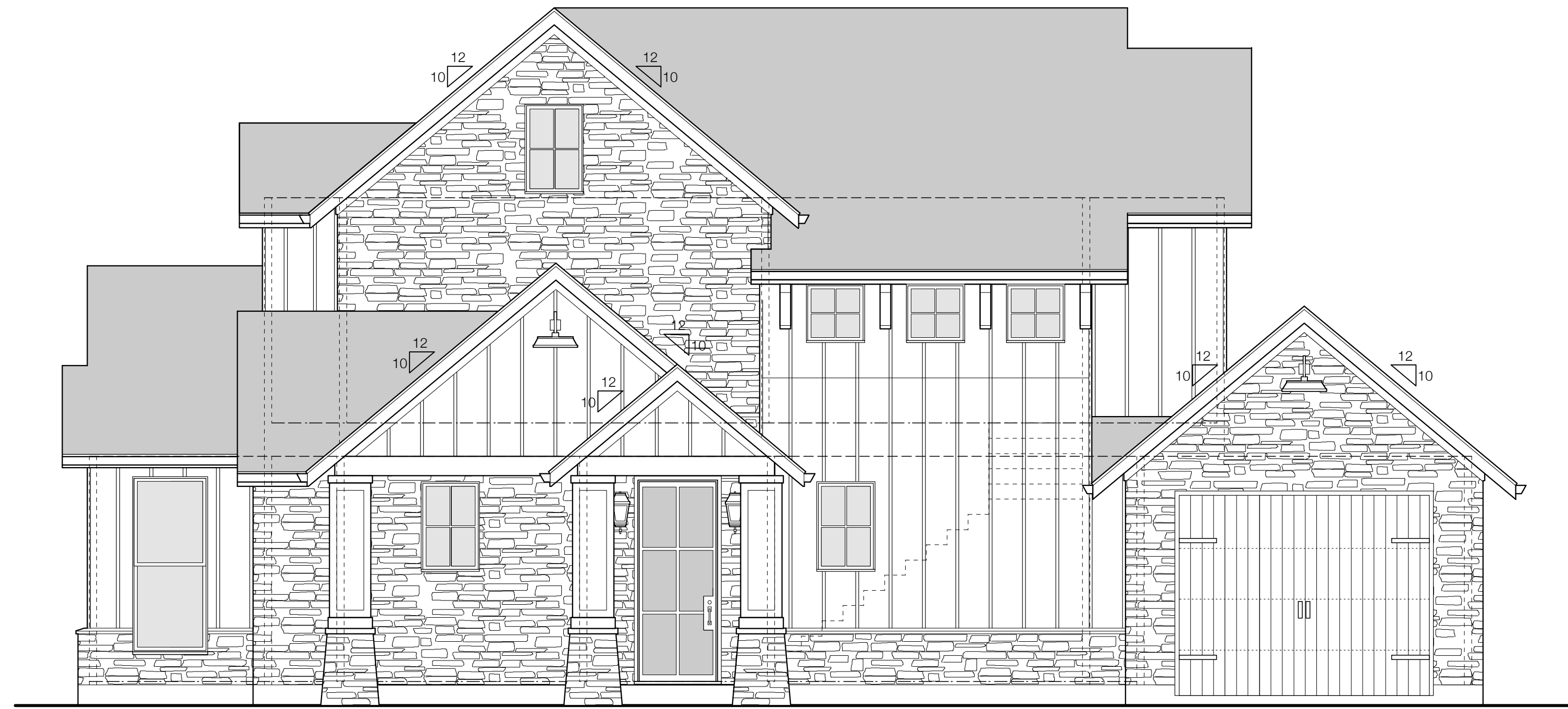
01 3.01 GUEST HOUSE EXTERIOR ELEVATION - FRONT Scale: 1/4" = 1'-0"
