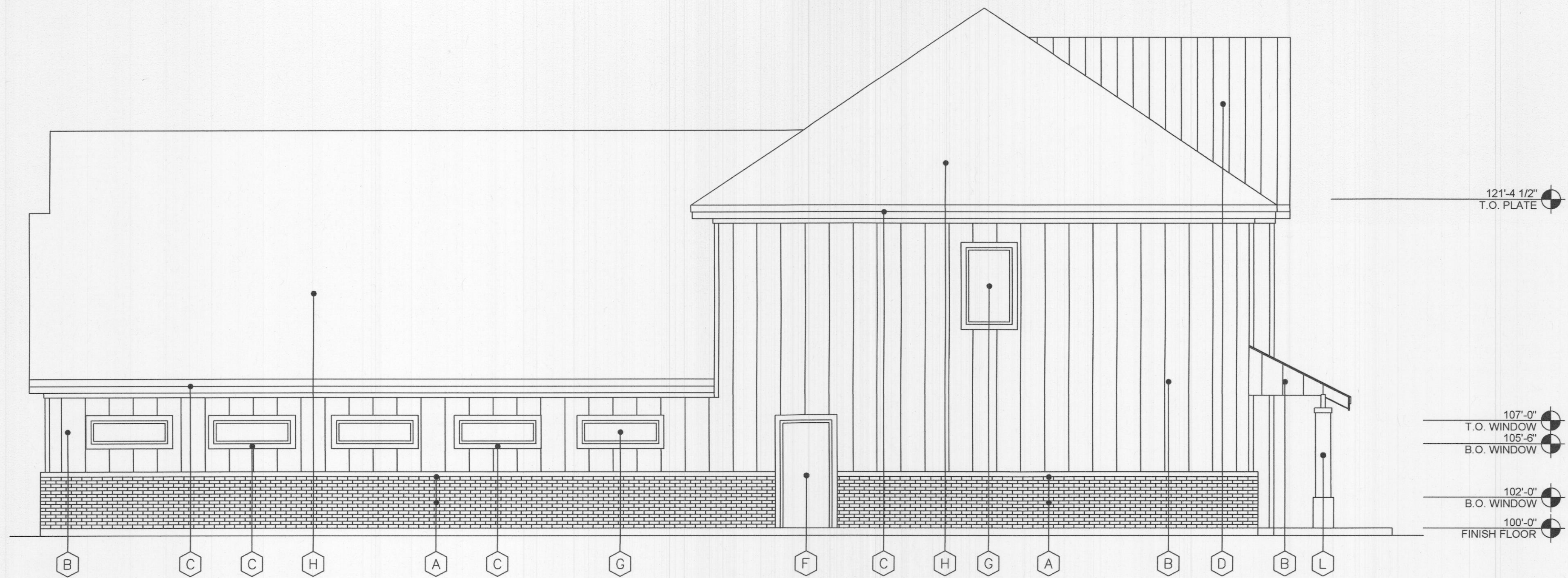
4 NORTH ELEVATION - MASONRY: 30% SCALE: 3/16" = 1'-0"
