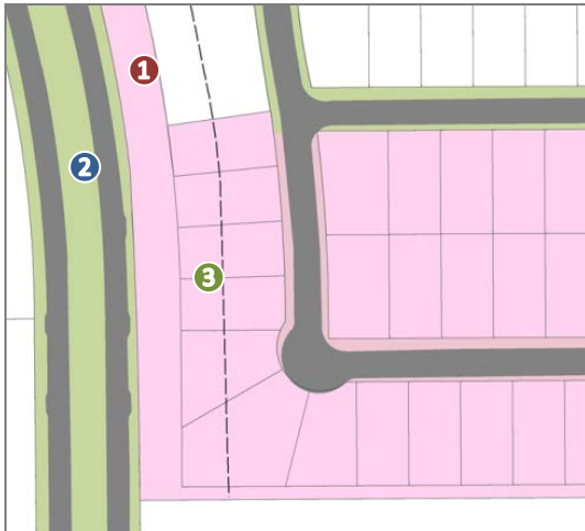
① : 50-Foot Landscape Buffer ② : John King Boulevard ③ : 50-Foot Rear Yard Building Setback
