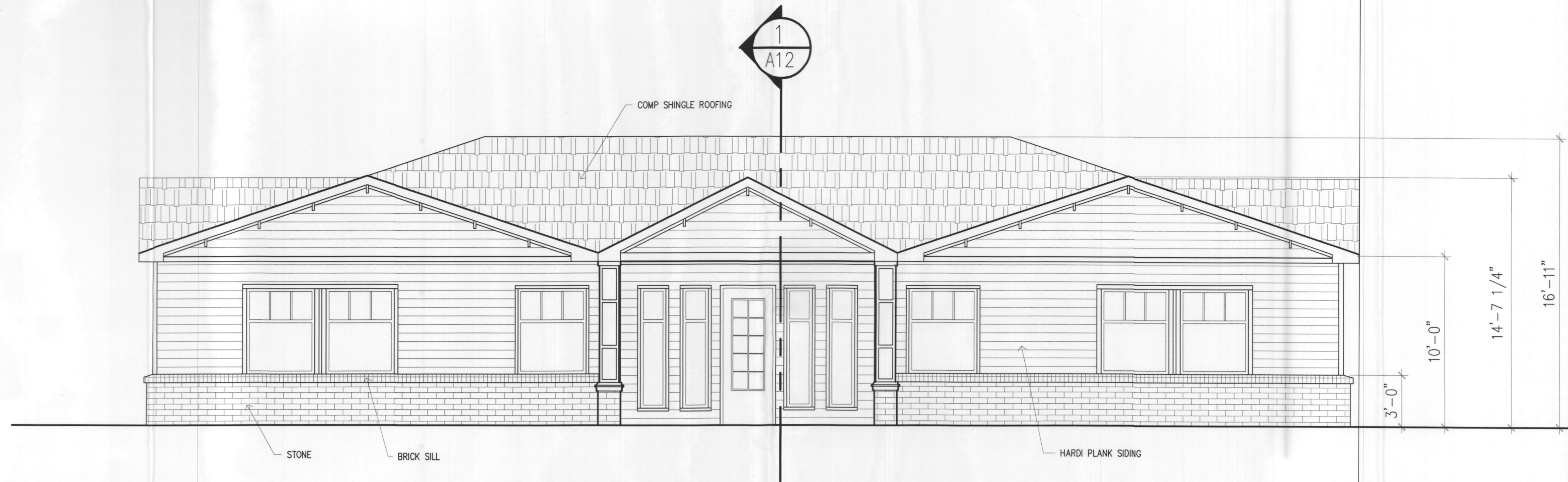
EAST ELEVATION 100% MASONRY 39% STONE 61% HARDI PLANK
