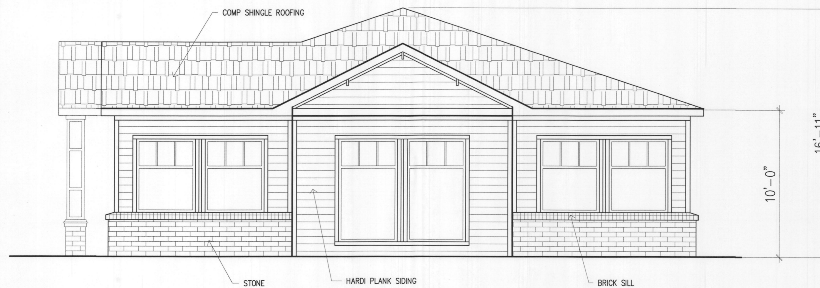
NORTH ELEVATION 100% MASONRY 34% STONE 66% HARDI PLANK
