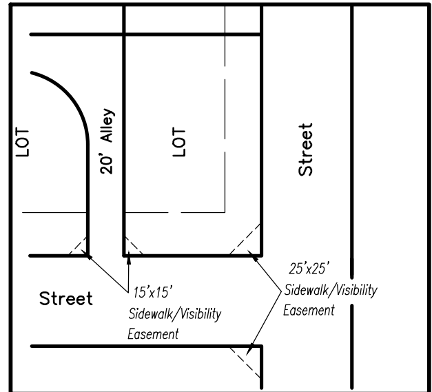
TYPICAL SIDEWALK/VISIBILITY EASEMENT DETAIL
