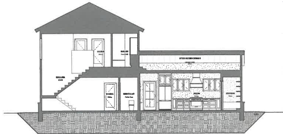
02 | BUILDING SECTION AT KITCHEN AND STAIRS 302 (1) x 42'
