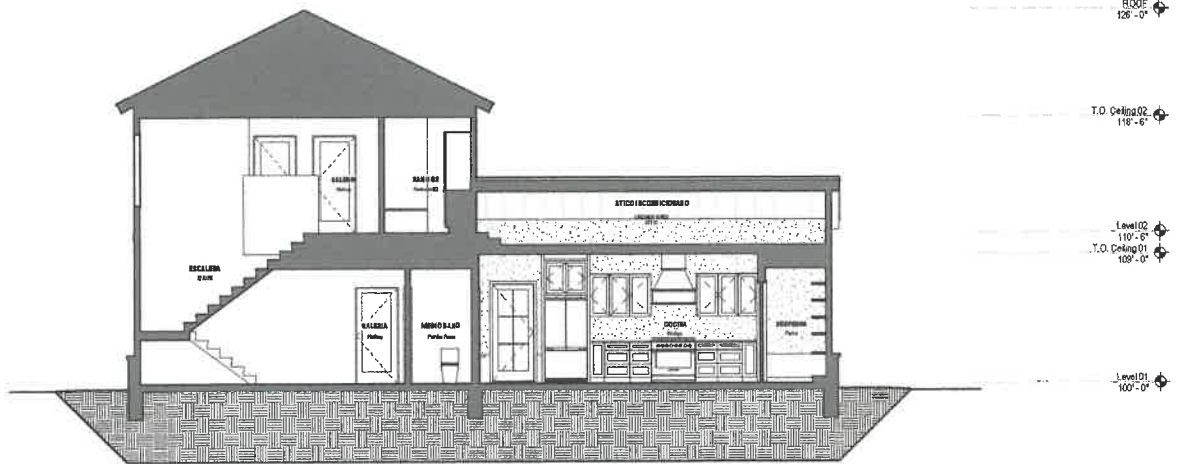
02 | BUILDING SECTION AT KITCHEN AND STAIRS
