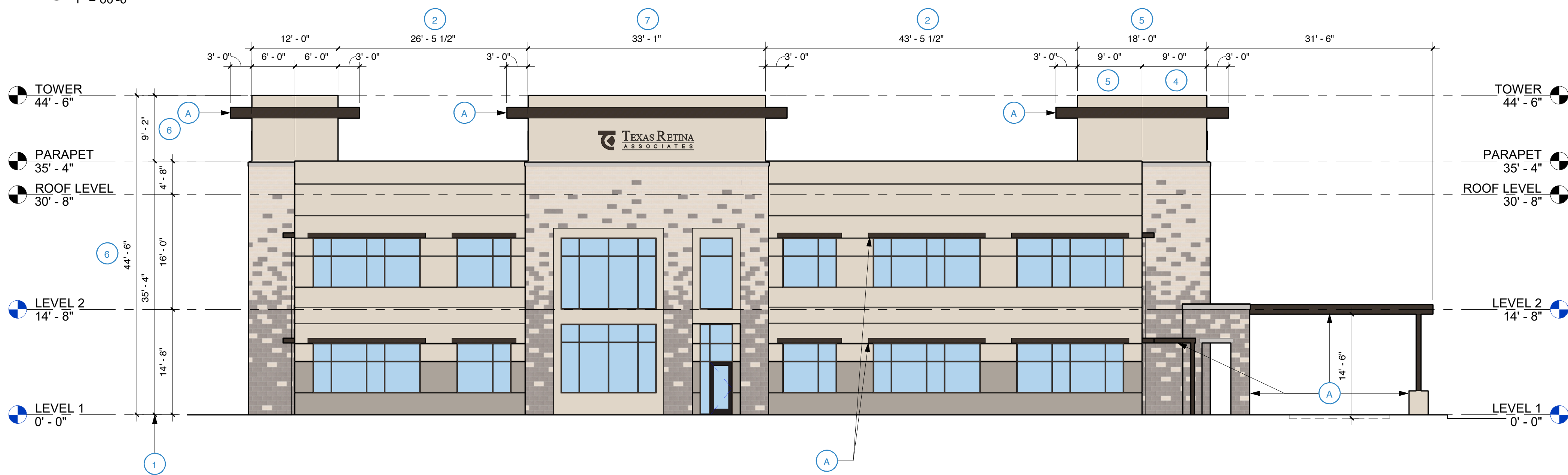
3 EAST ELEVATION (FACING RESIDENTIAL - PRIMARY FACADE) 1" = 10'-0"
