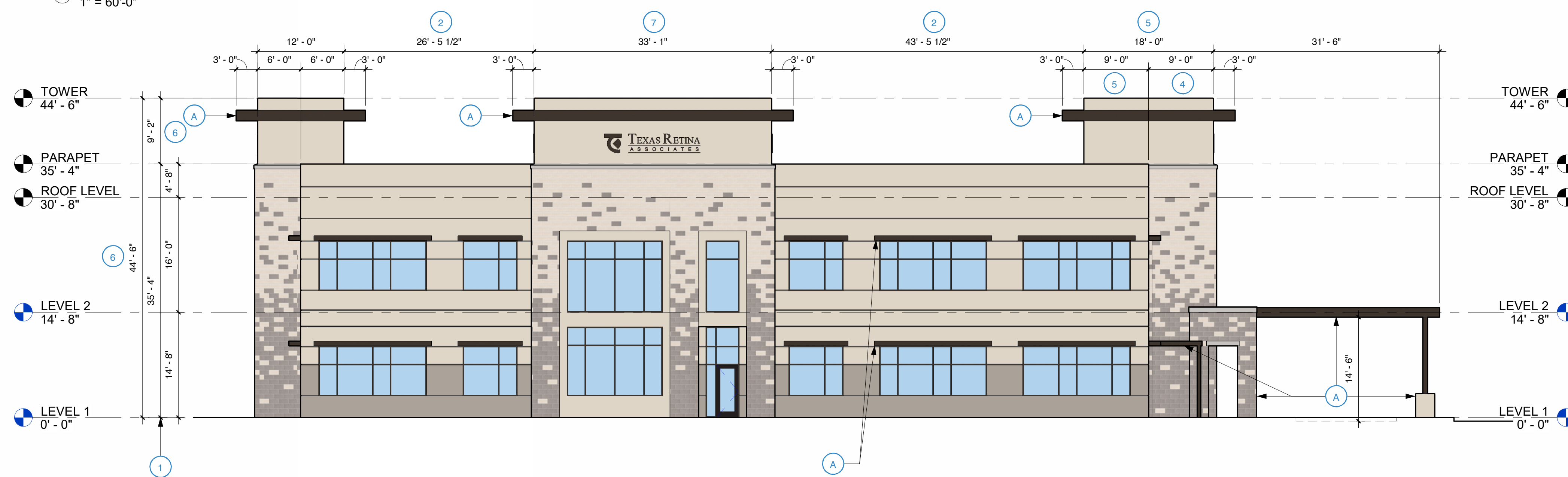
3 EAST ELEVATION (FACING RESIDENTIAL - PRIMARY FACADE) 1" = 10'-0"
