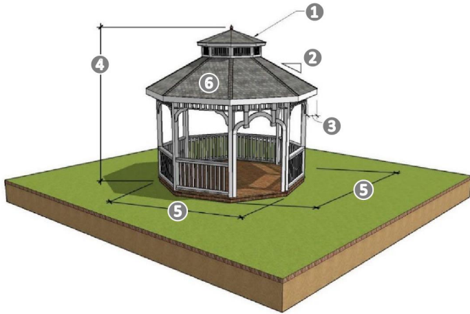
1: CUPOLA OR CLERESTORY; 2: 2:1 MINIMUM ROOF PITCH; 3: 1.5-FOOT MAXIMUM OVERHANG; 4: 18-FEET MAXIMUM HEIGHT WITH A CUPOLA OR CLERESTORY AND 15-FEET WITHOUT A CUPOLA OR CLERESTORY; 5: 12-FEET MAXIMUM; 6: ROOF CAN MATCH THE PRIMARY STRUCTURE OTHERWISE THE ROOF SHALL BE STANDING SEAM METAL.
