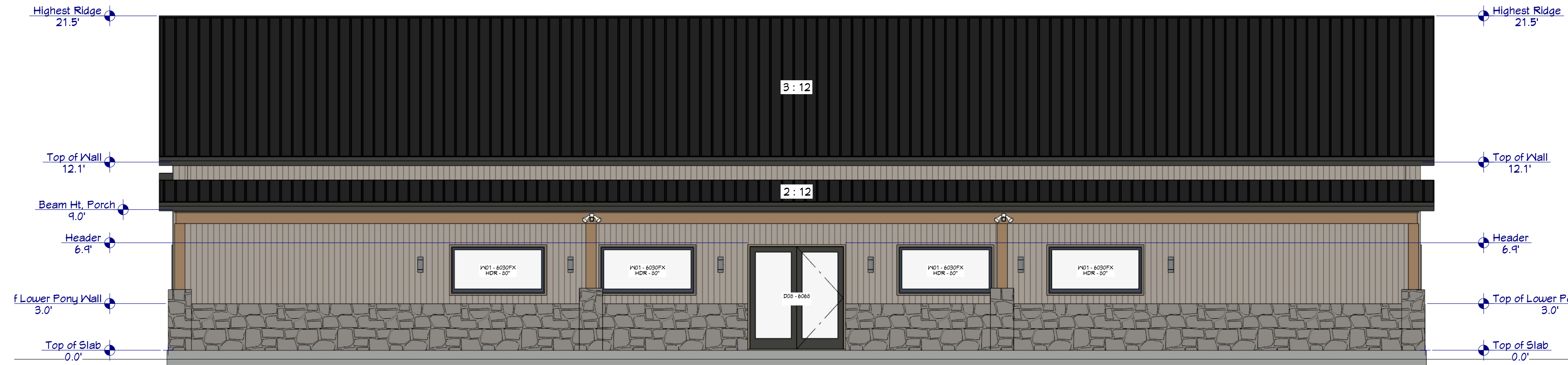
Exterior Elevation Front MATERIALS (EXCLUDES DOORS/WINDOWS & ROOF): R PANEL: 429 SF STONE PONY WALL: 245 SF
