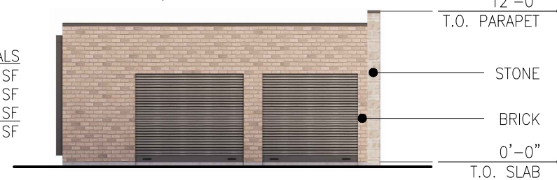
BLDG C SOUTH ELEVATION SCALE: 3/32" = 1'-0"
