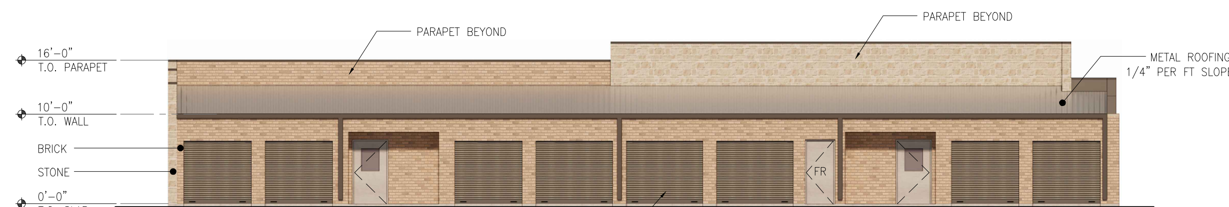
BLDG D NORTH ELEVATION SCALE: 3/32" = 1'-0"
