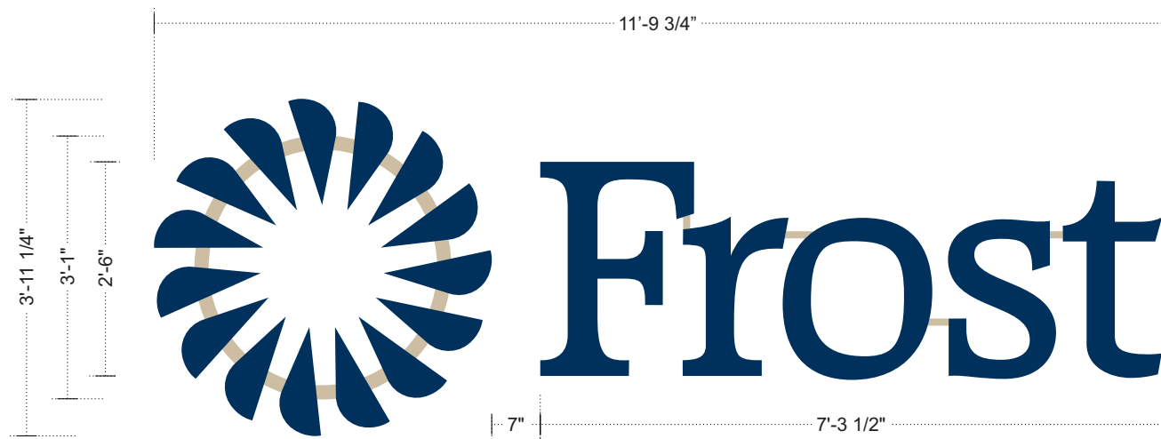
005 ICL.30 - ILLUMINATED CHANNEL LETTERS SCALE: 1/2" = 1' - QTY 1 34 SQ. FT.
