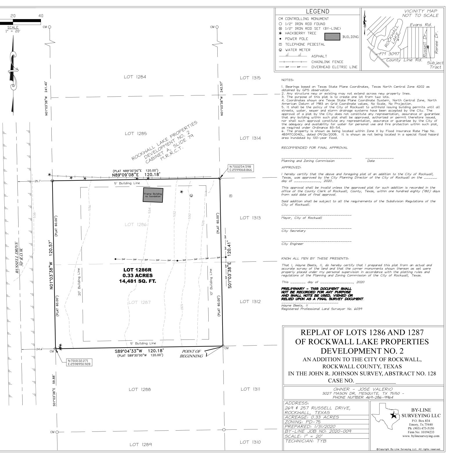
PntNo Bearing Distance Northing Easting Description 7010134.21 2599071.10 S  $89^{\circ}04'33'' W 120.18$ 7010132.27 2598950.93 N  $01^{\circ}03'38'' W 120.57$ 7010252.82 2598948.70 N  $89^{\circ}09'08'' E 120.18$ 7010254.60 2599068.87 S  $01^{\circ}03'38'' E 120.41$ 7010134.21 2599071.10 Closure Error Distance> 0.0000 Total Distance Inversed> 481.35
