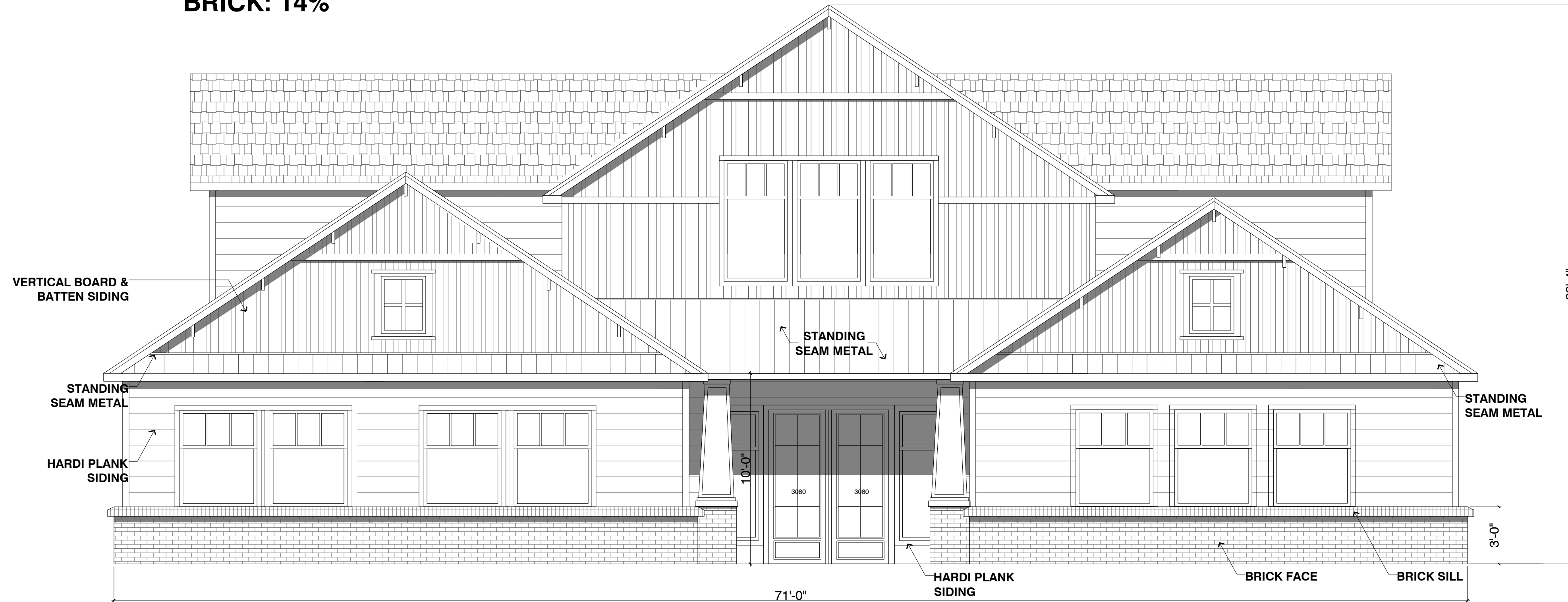
EAST ELEVATION: GOLIAD FRONTAGE
