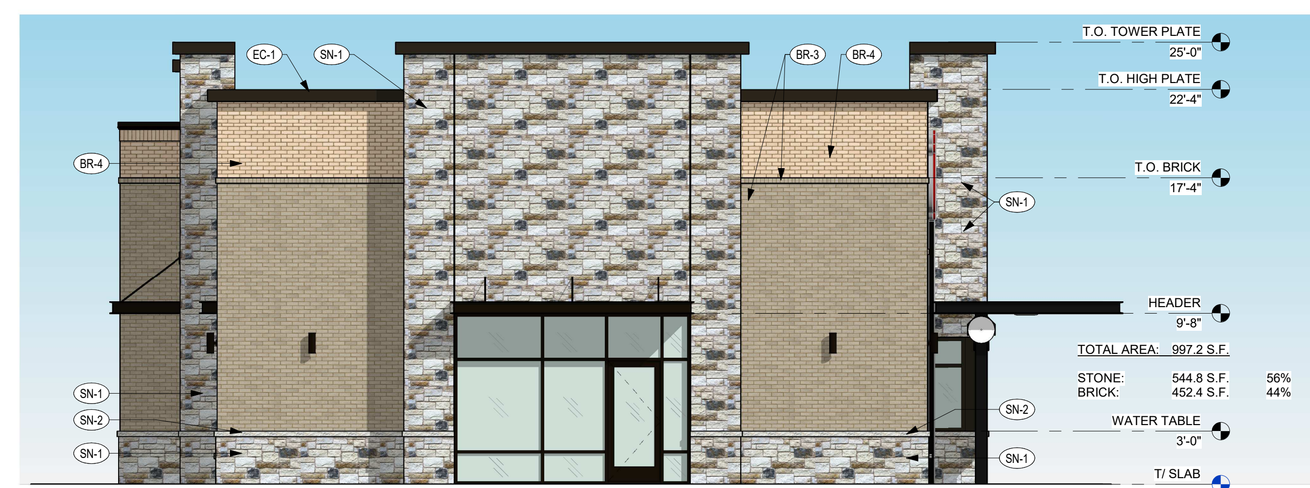
B4 EAST ELEVATION (FACING N. GOLIAD) 3/16" = 1'-0"
