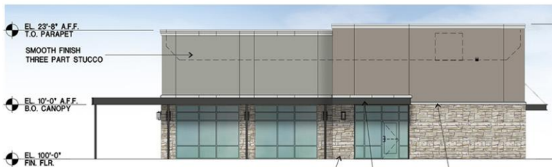
SIDE ELEVATION (MAIN ENTRY)
