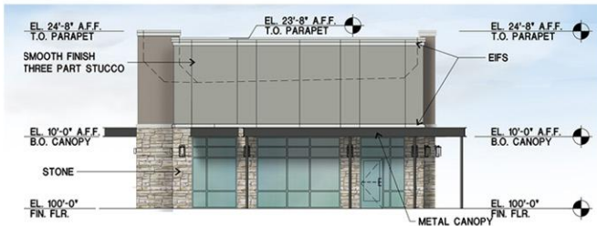
FRONT ELEVATION (FACING SH 205)
