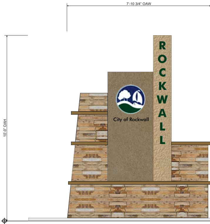
Front Elevation & Side Detail - Custom Monument Sign Structure - Sign B
