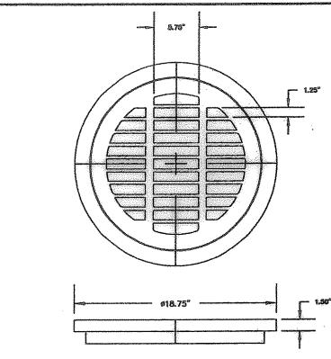
ROOF DRAIN DETAILS AS SHOWN
