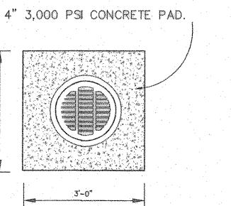
18" CAST IRON GRATE ROUND OR SQUARE DRÁINAREA = 161.4 SQ. INCH GRATE HAS H-20 (HEAVY TRAFFIC) DOT RATING QUALITY: MATERIAL SHALL CONFORM TO ASTM A48 - CLASS 30B
