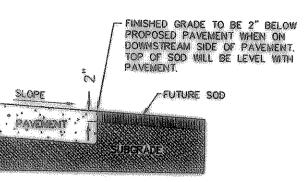
GRADING DETAIL FOR PAVEMENT WITHOUT CURB
