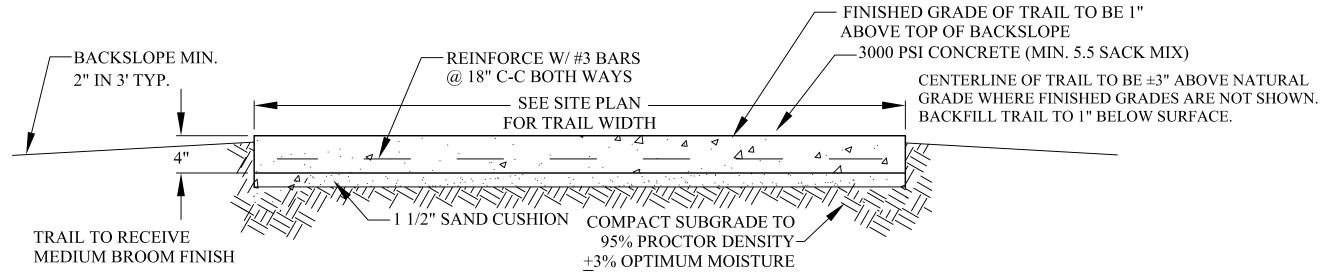
NOTES: CROSS SLOPE OF TRAIL TO BE ±1% WITH TERRAIN BUT NOT TO EXCEED 2%. RUNNING SLOPE OF TRAIL TO BE LESS THAN 5% IN ALL AREAS.
