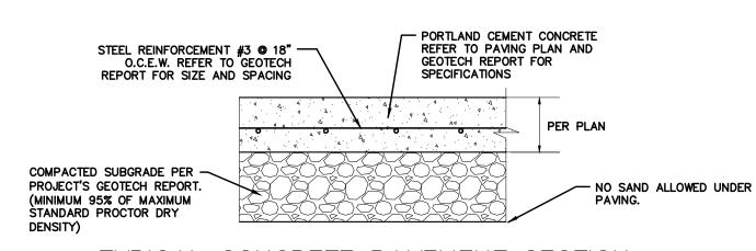
TYPICAL CONCRETE PAVEMENT SECTION
