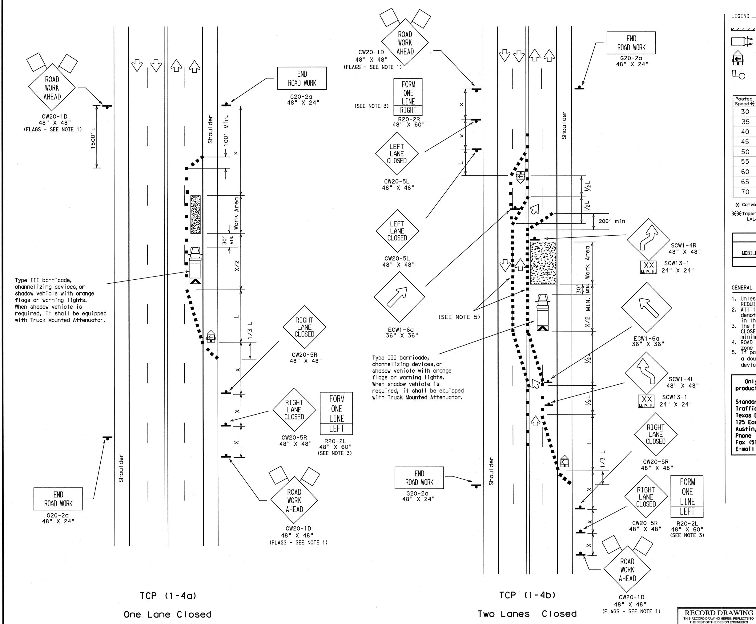
■ Channelizing Devices Type III Barricade Truck Mounted Attenuator Heavy Work Vehicle Portable Changeable
