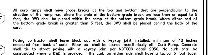
All work associated with accessible routes shall be installed flush with all features to minimize vertical surface discontinuities. Each segment along accessible route shall be flush with no more (zero tolerance) than a 1/4-inch grade separation (elevation difference), or 1/2-inch grade separation if beveled (bevel slope shall not be steeper than 50%).
