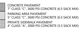
NOTE: CONCRETE PAVEMENT & PARKING AREA PAVEMENT TO HAVE #4 BARS ON 18" CTRS. BOTH WAYS
