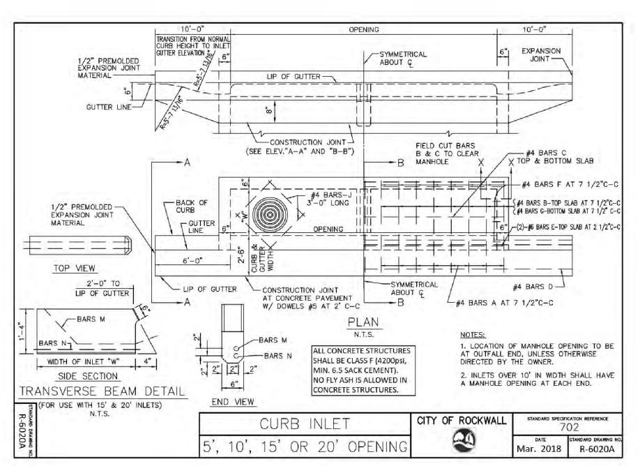
I. ALL CONCRETE FOR STRUCTURES SHALL BE CLASS F (4200 PSI, MINIMUM 6.5 SACK CEMENT). 2. NO FLY ASH IS ALLOWED IN CONCRETE FOR STRUCTURES
