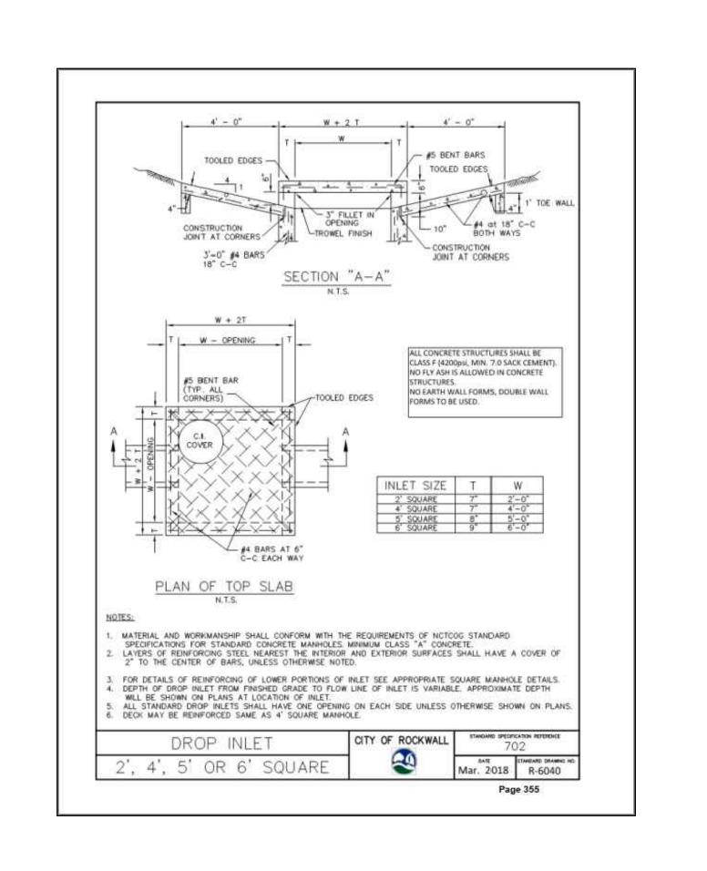
Note: All materials and construction shall be in accordance with the City of Rockwall Standard Specifications and Construction Standards, and Standard Specifications for Public Works Construction prepared by North Central Texas Council of Governments (Latest Revision), and to the regulations of The Texas Commission on Environmental Quality.
