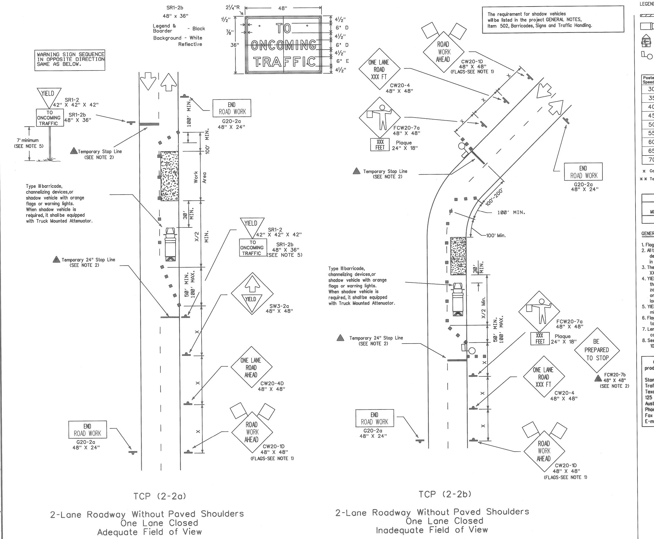
2-Lane Roadway Without Paved Shoulders One Lane Closed Inadequate Field of View
