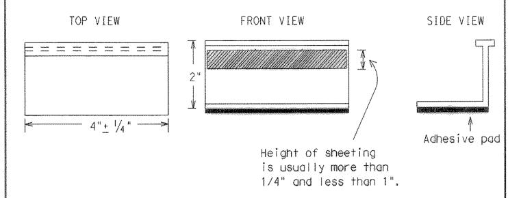
STAPLES OR NAILS SHALL NOT BE USED TO SECURE TEMPORARY FLEXIBLE-REFLECTIVE ROADWAY MARKER TABS TO THE PAVEMENT SURFACE
