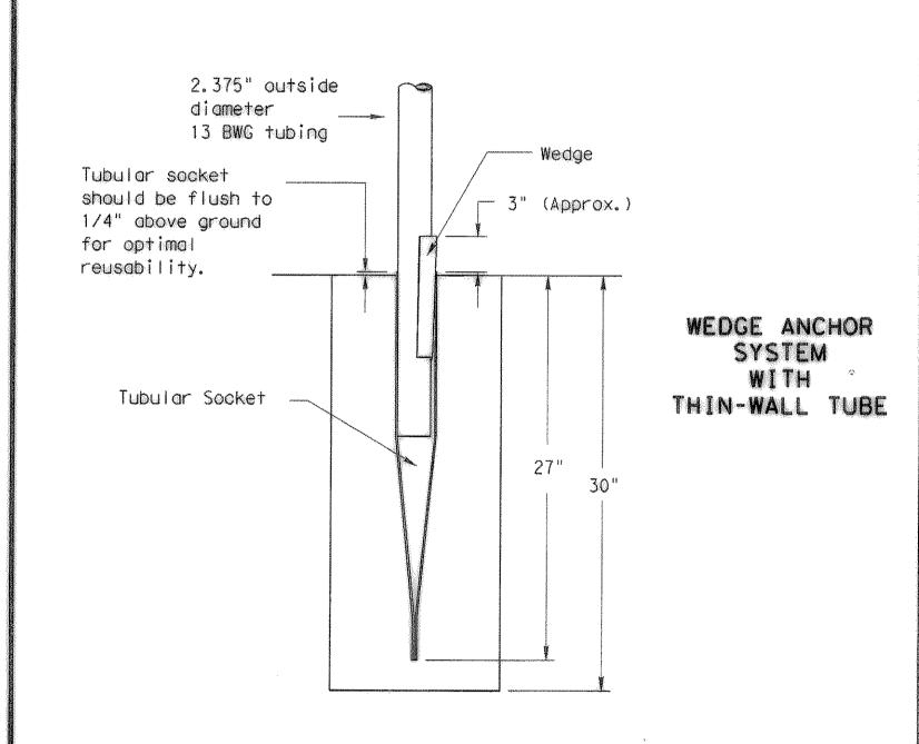
The wedge anchor system with thin wall tubing may be used to support up to 10 sq. ft. of sign area.
